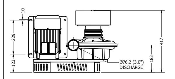
Siemens AC Induction Motor, IE3, 1.5kW P/N:1LE1003-0EA02-2NB4-Z F74+Y58 {Y58:D024 E055}
